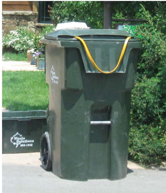
Fig. A5. Rubber sling—Bear-resistant garbage containers secured by a heavy-duty, rubber sling that is stretched over a molded lip. This container was often not secured likely because too much garbage prevented the rubber sling to be properly secured.
