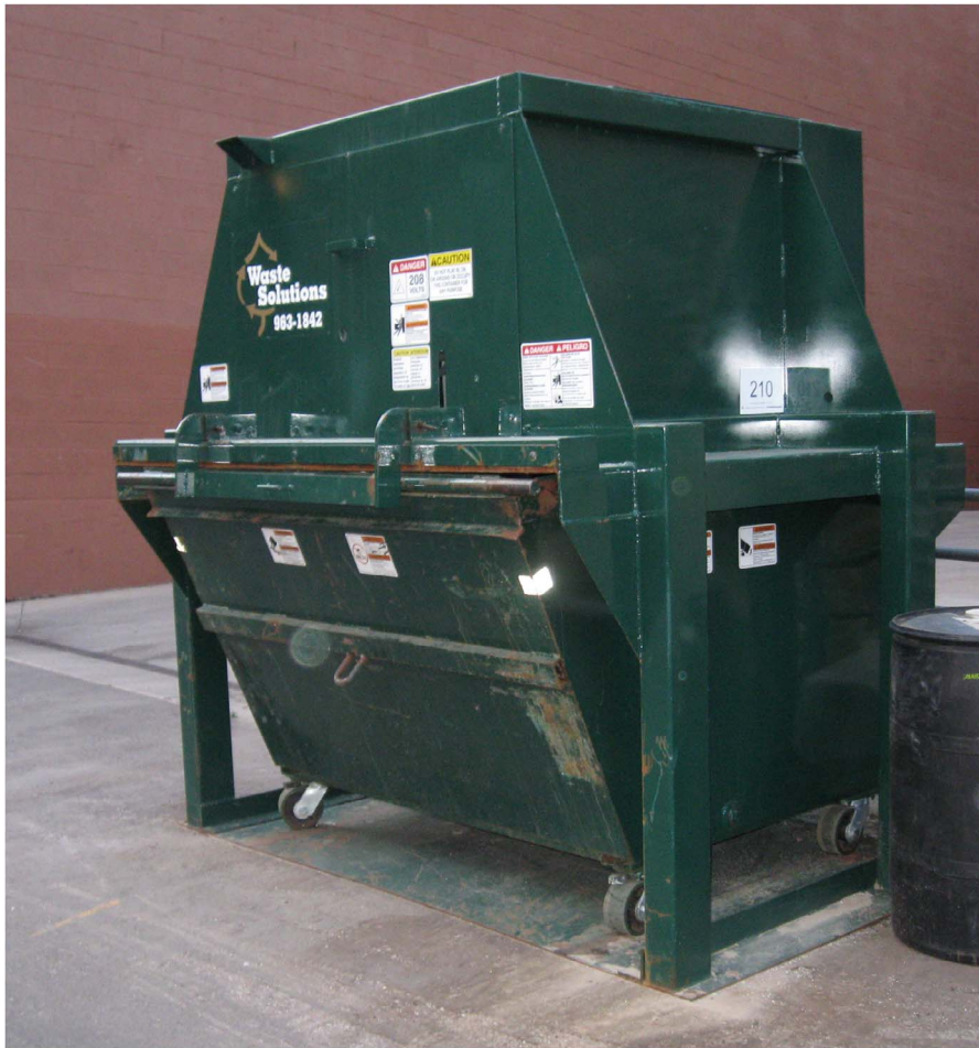
Fig. A6. Compactor—Bear-resistant garbage containers secured when a compacting mechanism is locked over the dumpster. These containers are robust, but often had trash placed next to the compactor suggesting that the design of the compacting mechanism may be difficult for some users to operate.
